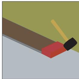
The end joints of this product features an integrated click-locking system with pushdown technology for an easy and speedy installation. Align the tongue and groove on the end joint of the next piece and press down.
