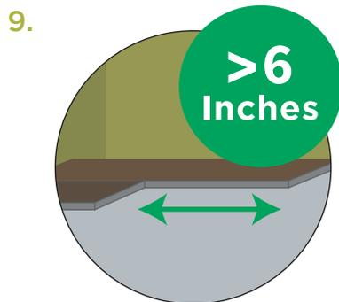
9. Maintain proper spacing (at least 6" for planks, and equal to half its length for tiles) between end joints for best appearance.
