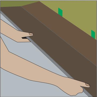
Position the first board in place by angling it up slightly, pushing forward and interlocking the side tongue. The long side of the plank or tile **MUST BE SNUG** against the adjoining plank or tile with **NO GAPPING**. If everything is aligned correctly, there will be a slight click from the end joint as the panel is successfully engaged and reaches its final position after being lowered into place.
