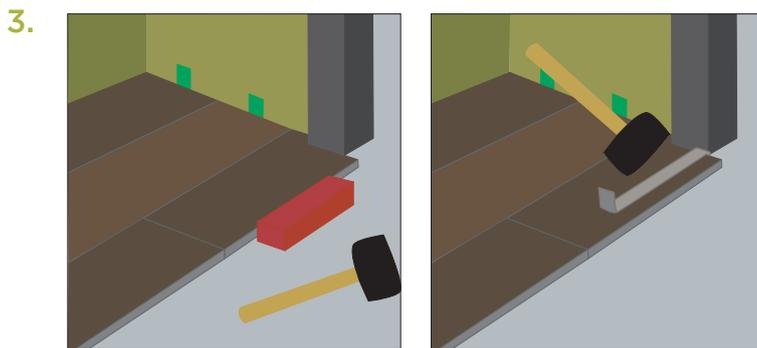
After the groove ledge has been trimmed, place the board in place and tighten with a pull bar. The installer must be sure that the required expansion gap has been maintained and the flooring is not pinched.
