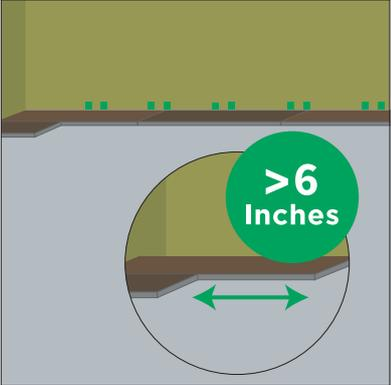
For tile installations, begin the second row with a half tile. For plank installations, if the cut plank is at least 6” in length, use it to begin the second row. If the cut plank is shorter than 6” do not use it. Instead, begin with a new board that is at least 6” in length and allows 6” between the end joints on the adjacent planks. End joint spacing for tiles should always be equal to a half tile.
