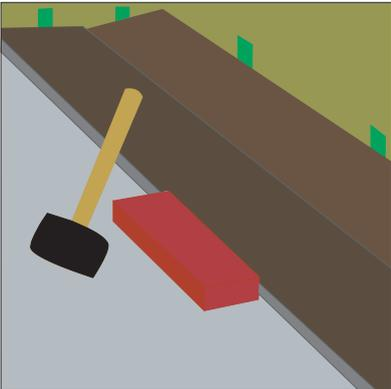
Tap the joint with the rubber mallet using a downward angle striking motion towards the adjoining end joint until the tongue and groove lock together on the side and ends.
