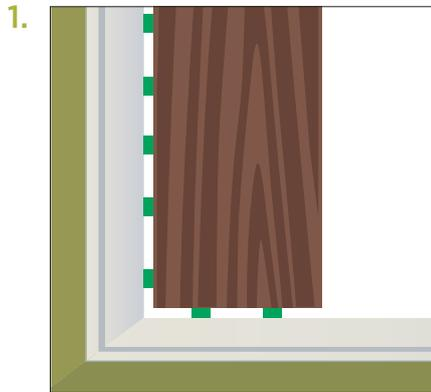
Starting from the left with the tongue-side facing the wall, carefully place the first board in place, using spacers to leave a ¼" expansion gap between the wall and edges of the plank or tile.
